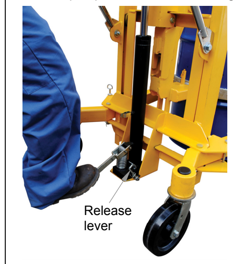
Press foot pump treadle to raise carriage
